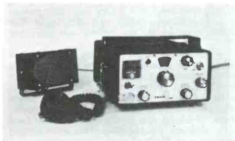
The Tram XL-100 CB Transceiver shown with its separate speaker. A snap-on clamp at each side of the set allows it to be quickly installed or removed from the gimbal bracket mount.
